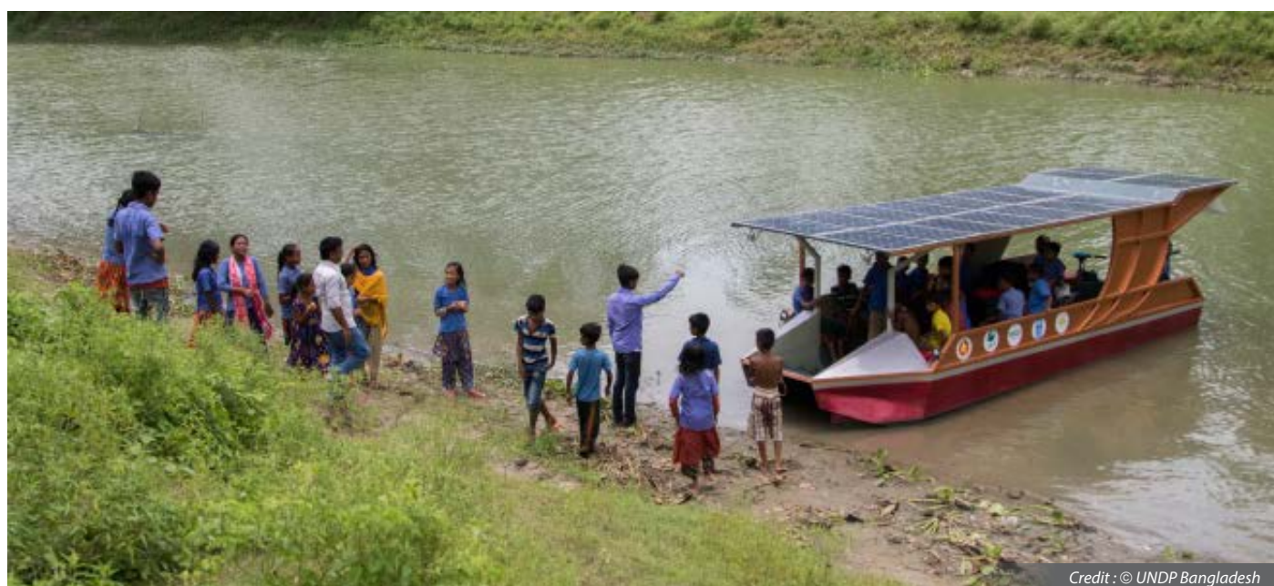
A locally built environment friendly solar engine boat, which can be used for carrying school children or as rescue boat in flood affected areas.
